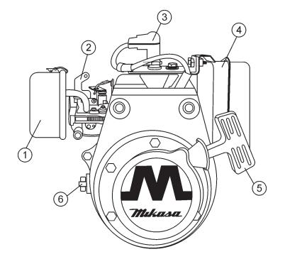
Figure 3. Robin EH-12-2D Engine Controls and Components
